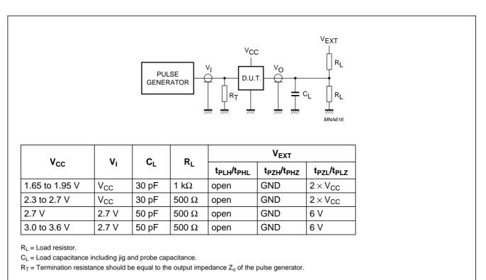
Fig.6 Load circuitry for switching times.
