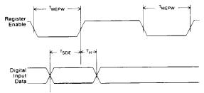
Digital Data Hold Time from Register Enable is Onsec.
