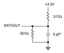
Figure 2. Output Load
