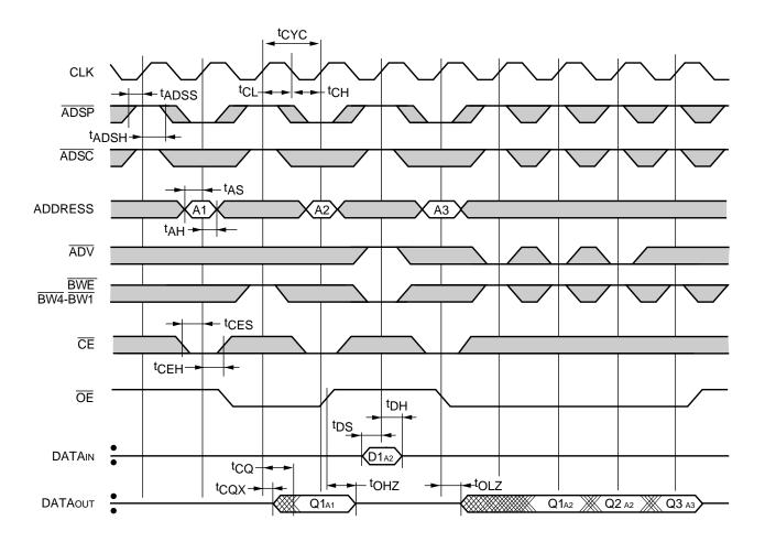
NOTES: 1.  $\overline{\text{CE2}}$  and CE2 have timing identical to  $\overline{\text{CE}}$ . On this diagram, when  $\overline{\text{CE}}$  is low,  $\overline{\text{CE2}}$  is low and CE2 is high. When  $\overline{\text{CE}}$  is high and CE2 is low.
