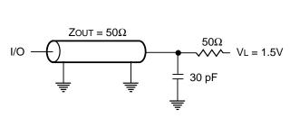
Figure 1. Output Load
