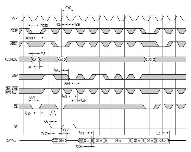
NOTES: 1. Qn(A2) refers to output from address A2. Q1-4 refers to outputs according to burst sequence.
