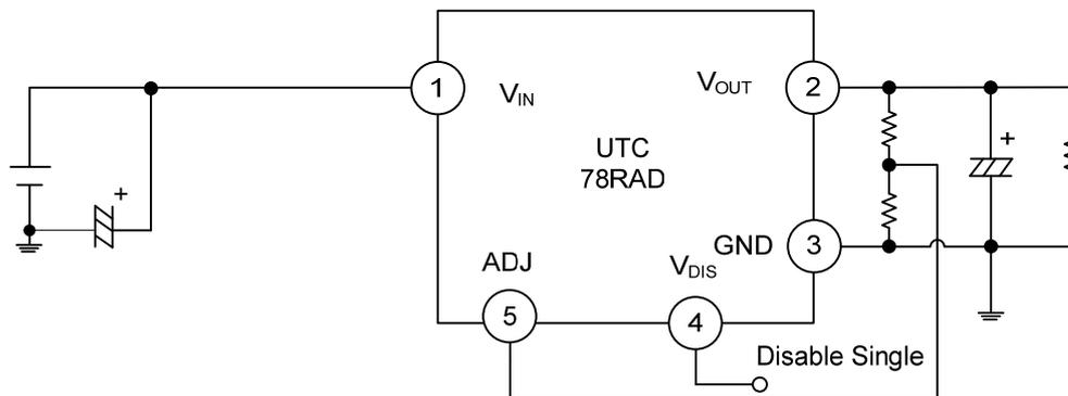
\*  $C_i$  is required if regulator is located an appreciable distance from power supply filter. [ $C_i > 0.33\mu\text{F}$  (Electrolytic)]
