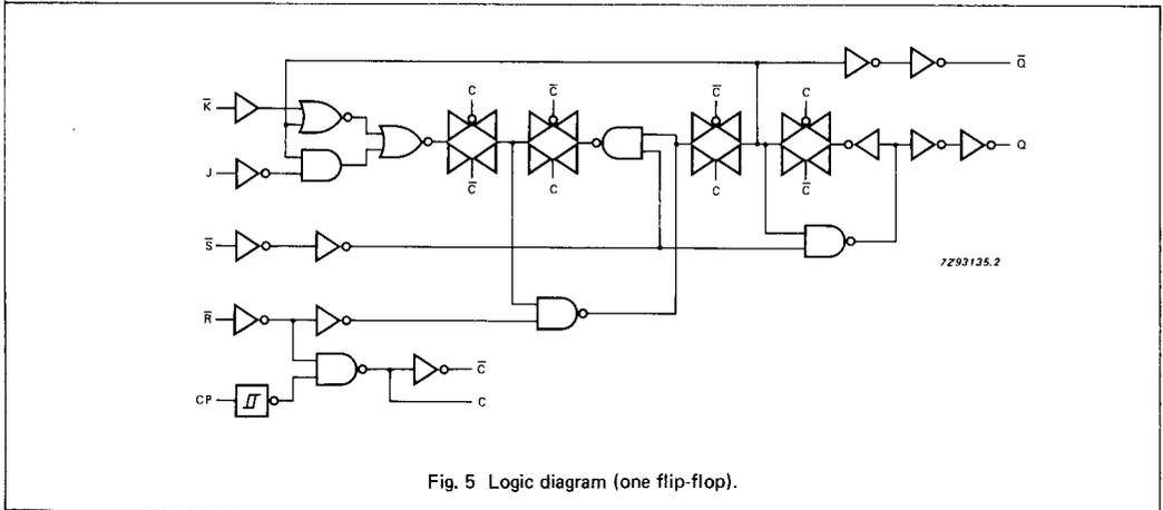
Fig. 5 Logic diagram (one flip-flop).
