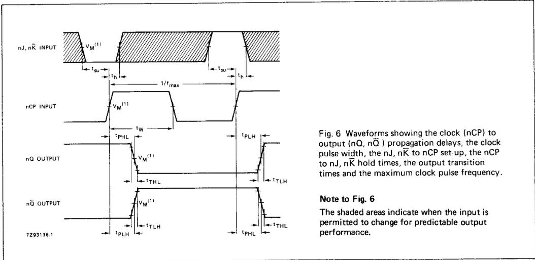
Fig. 6 Waveforms showing the clock (nCP) to output (nQ, nQ-bar) propagation delays, the clock pulse width, the nJ, nK to nCP set-up, the nCP to nJ, nK hold times, the output transition times and the maximum clock pulse frequency.
