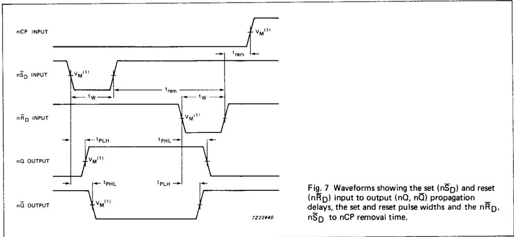
Fig. 7 Waveforms showing the set (nSD-bar) and reset (nRD-bar) input to output (nQ, nQ-bar) propagation delays, the set and reset pulse widths and the nSD-bar, nRD-bar to nCP removal time.
