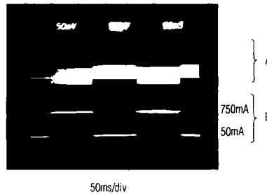
A: V_{out} , 50mV/DIV, DC-COUPLED B: I_{out} , 500mA/DIV, 50mA TO 750mA CIRCUIT OF FIG. 3, V_+ = 12V , T_A = +25^\circ C
