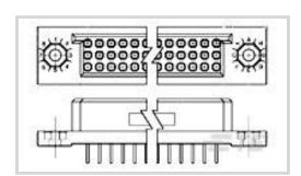
PCB Connector Assembly Type: PCB Mount Receptacle
