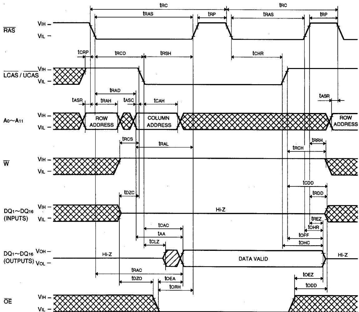
Note 30: Early write, delayed write, read write or read modify write cycle is applicable instead of read cycle.
