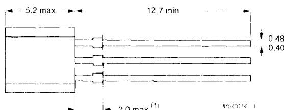
Note (1) Terminal dimensions within this zone are uncontrolled to allow for flow of plastic and terminal irregularities.
