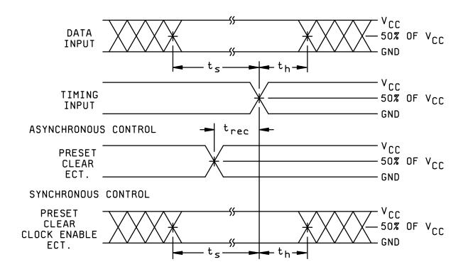
FIGURE 4. Switching waveforms and test circuit.
