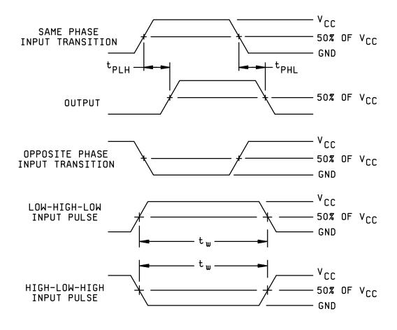
FIGURE 4. Switching waveforms and test circuit - Continued.
