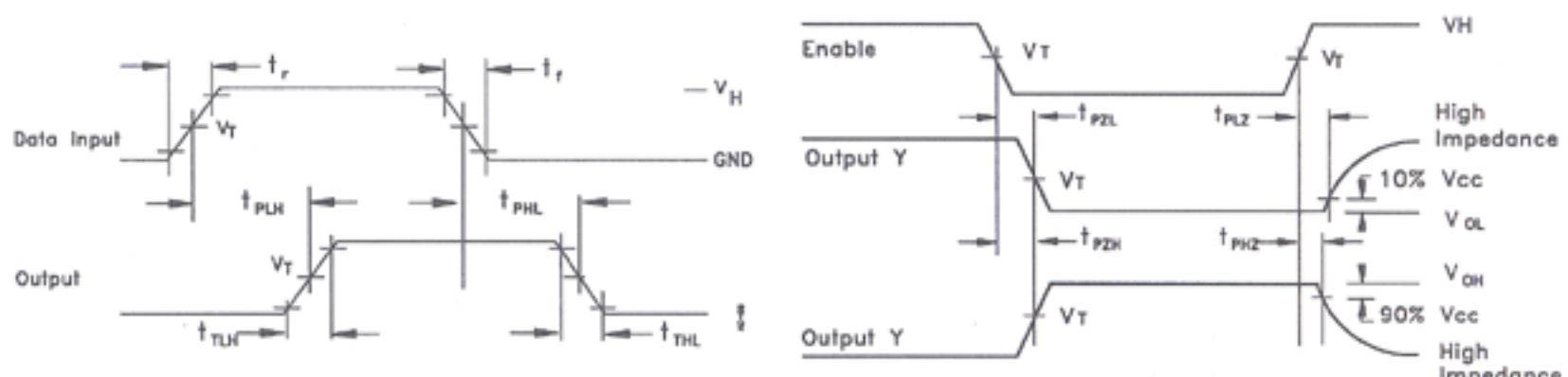
Input threshold Voltage, V<sub>T</sub> = 50% V<sub>CC</sub> for HC, 1.3V for HCT
