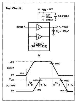
Figure 2. Non-inverting Driver Switching Time
