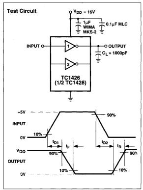
Figure 1. Inverting Driver Switching Time
