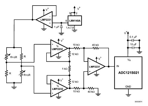
FIGURE 5. Strain Gauge Bridge Amplifier
