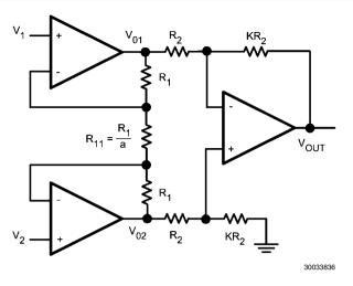
**FIGURE 3. Instrumentation Amplifier**
