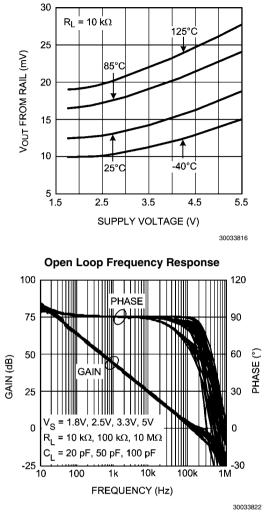
**Output Swing Low vs. Supply Voltage**
