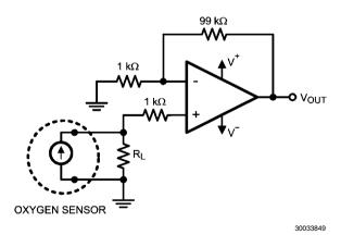
FIGURE 6. Precision Oxygen Sensor
