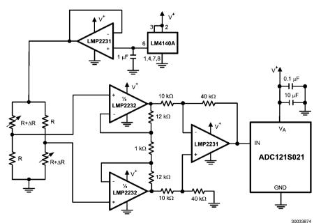
Strain Gauge Bridge Amplifier
