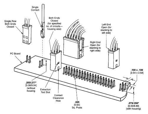
\*If post is longer than maximum specified, post tip may butt against wire ends.
