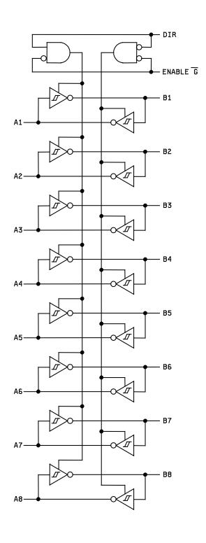
FIGURE 3. Logic diagram.
