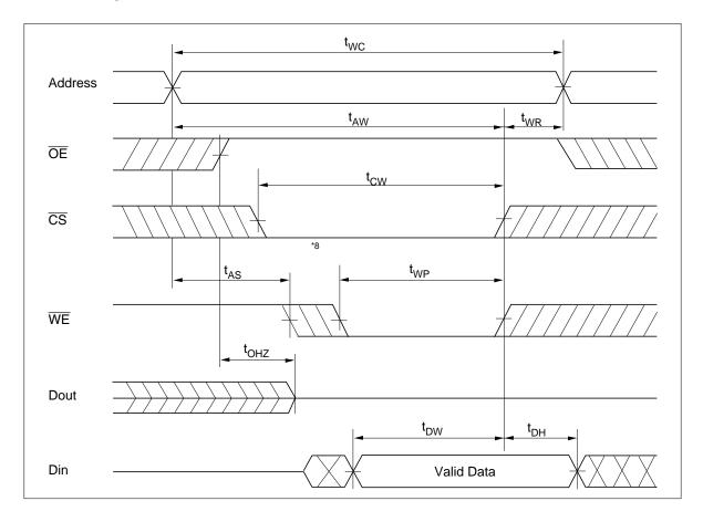
Write Timing Waveform (2)  $(\overline{OE} Low Fixed)$
