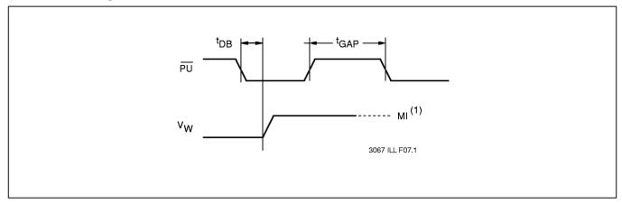
Notes: (1) MI in the A.C. timing diagram refers to the minimum incremental change in the wiper voltage.
