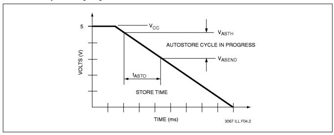
$\begin{tabular}{lll} \textbf{Notes:} & V_{ASTH}-AUTOSTORE \ threshold \ voltage \\ & V_{ASEND}-AUTOSTORE \ cycle \ end \ voltage \\ \end{tabular}$
