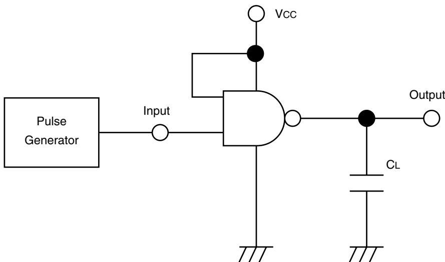
Note: open output when measuring supply current
