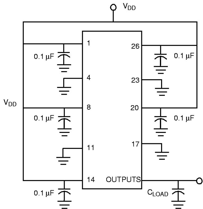
Note: All capacitors should be placed as close to each pin as possible.
