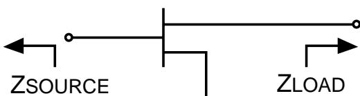
Z<sub>SOURCE</sub> = Impedance of the input circuit as seen by the gate
