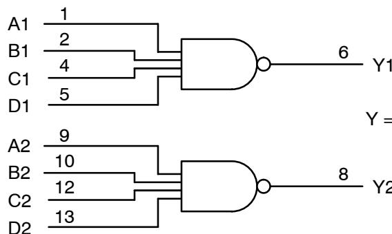
$$Y = \overline{A} \cdot \overline{B} \cdot \overline{C} \cdot \overline{D} \text{ or } Y = \overline{A} + \overline{B} + \overline{C} + \overline{D}$$
