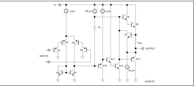
Figure 2. Equivalent schematic.
