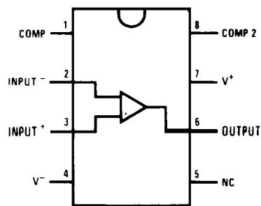
\*Package is connected to Pin 4 (V-)
