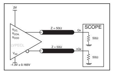
3.3V LVPECL Output Load AC Test Circuit
