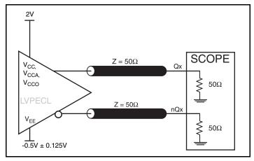
2.5V LVPECL Output Load AC Test Circuit
