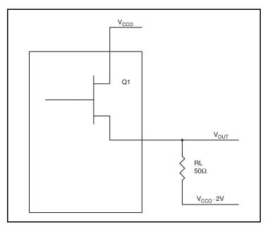
Figure 7. LVPECL Driver Circuit and Termination
