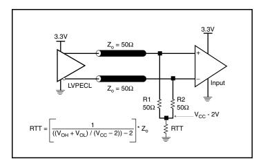
Figure 4A. 3.3V LVPECL Output Termination
