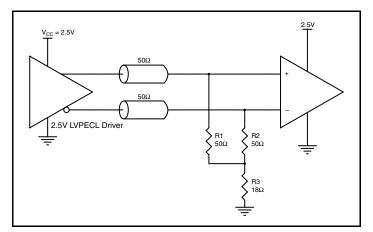
Figure 5B. 2.5V LVPECL Driver Termination Example
