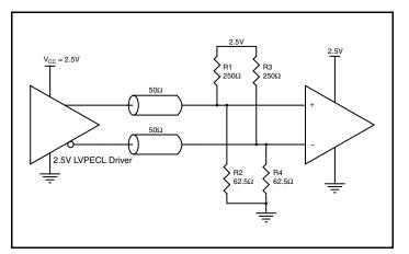
Figure 5A. 2.5V LVPECL Driver Termination Example
