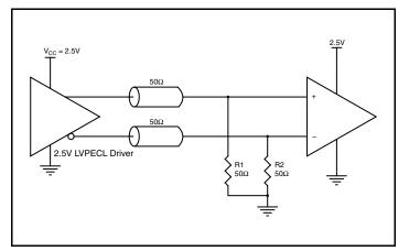
Figure 5C. 2.5V LVPECL Driver Termination Example
