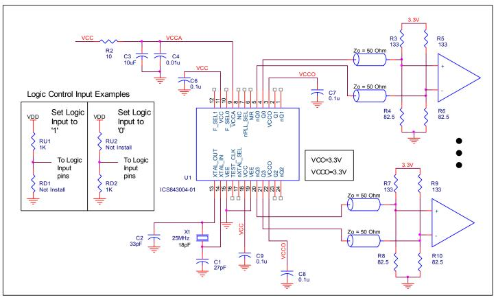
Figure 6. ICS843004I-01 Schematic Example
