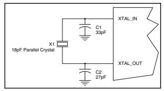
Figure 2. Crystal Input Interface
