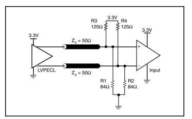
Figure 4B. 3.3V LVPECL Output Termination
