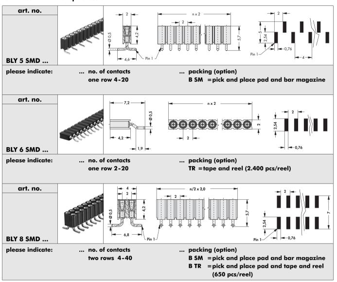
contact shell surface: tin-plated contact spring: gold-plated
