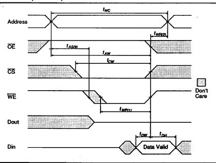
Write Cycle 2 Timing Waveform (OE Low Fixed)
