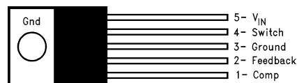
Figure 1. Top View Order Number LM2577T-12, LM2577T-15, or LM2577T-ADJ See NS Package Number T05A
