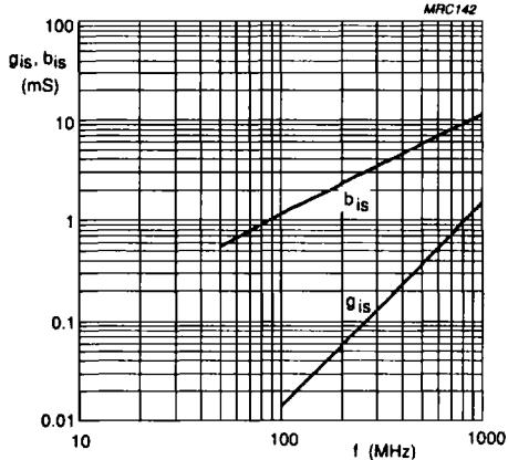
$V_{DS} = 10$  V;  $I_D = 1$  mA;  $T_{amb} = 25$  °C.
