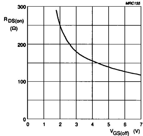
$V_{DS} = 100$  mV;  $V_{GS} = 0$ .
