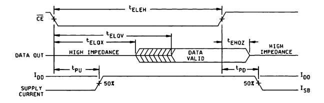
$\overline{\rm WE}$  is high for read cycle. Address valid prior to or coincident with  $\overline{\rm CE}$  transition low.
