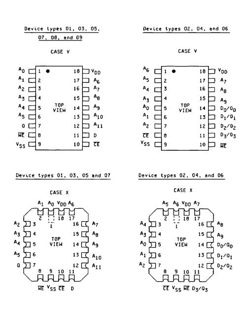
FIGURE 2. Terminal connections.
