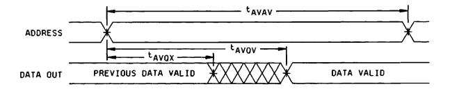
$\overline{\text{WE}}$  is high for read cycle. Device is continuously selected,  $\overline{\text{CE}}$  =  $\text{V}_{\text{IL}}$ .
