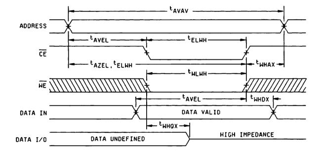
If CE goes HIGH simultaneously with WE HIGH, the output remains in a high impedance state.
