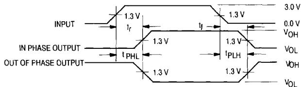
VOLTAGE WAVEFORMS ENABLE AND DISABLE TIMES,
