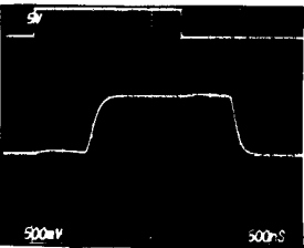
MUX-24 SMALL-SIGNAL SWITCHING WITH FILTERING AND 2.5µs SAMPLE TIME
