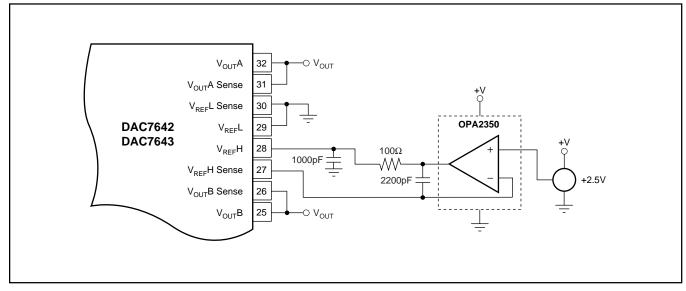
FIGURE 10. Single-Supply Buffered V<sub>REF</sub>H.
