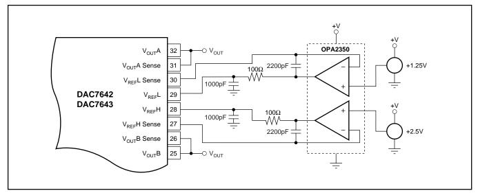
FIGURE 9. Single-Supply Buffered Reference with V<sub>REF</sub>L = +1.25V and V<sub>REF</sub>H = +2.5V.
