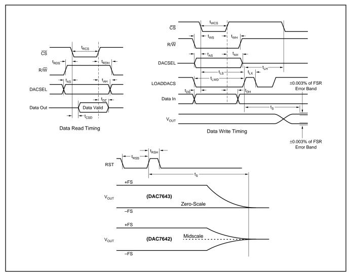
FIGURE 14. Digital Input and Output Timing.
