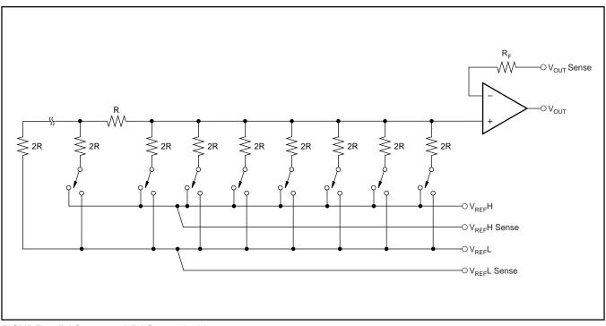
FIGURE 1. DAC7642 and DAC7643 Architecture.
