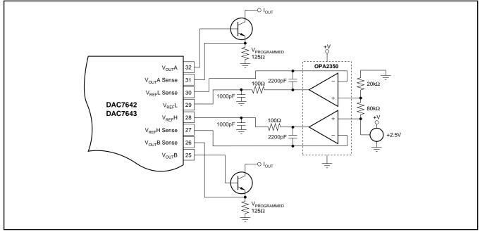
FIGURE 15. 4-20mA Digitally Controlled Current Source.
