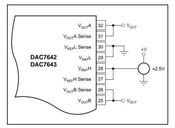
FIGURE 12. Low-Cost Single-Supply Configuration.
