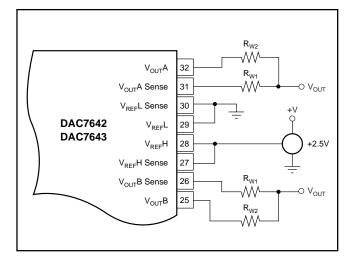
FIGURE 4. Analog Output Closed-Loop Configuration. R<sub>W</sub> represents wiring resistances.
