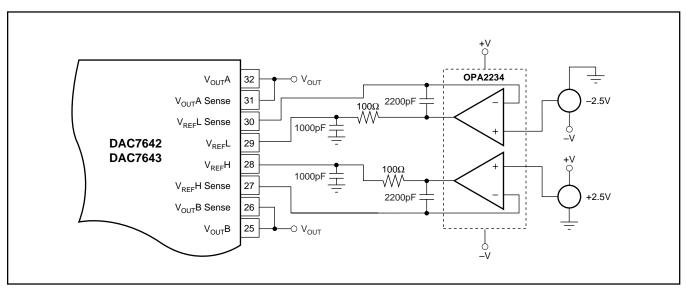
FIGURE 5. Dual Supply Configuration-Buffered References, Used for Dual-Supply Characteristic Curves.
