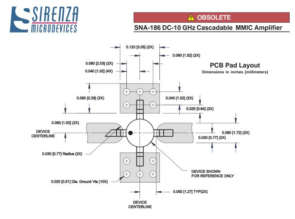
Nominal Package Dimensions Dimensions in inches [millimeters] Refer to drawing posted at www.sirenza.com for tolerances.
