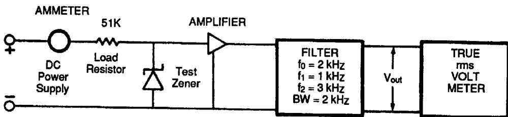
Noise is specified in microvolts per square root hertz. The maximum noise in a particular application may be calculated from the following equation:
