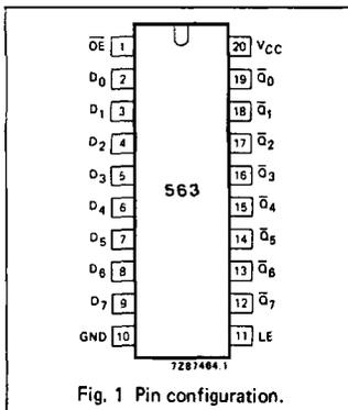
Fig. 1 Pin configuration.
