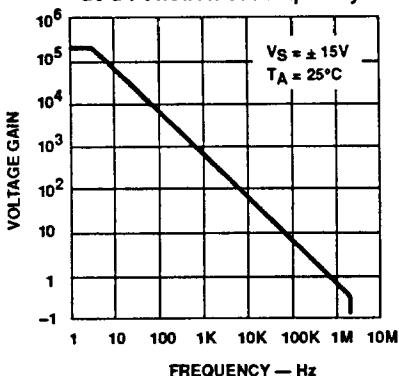
Open-Looped Voltage Response as a Function of Frequency
