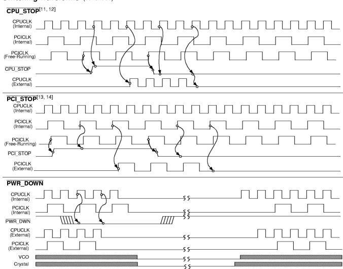
Shaded section on the VCO and Crystal waveforms indicates that the VCO and crystal oscillator are active, and there is a valid clock.
