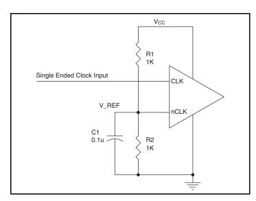
Figure 1. Single-Ended Signal Driving Differential Input
