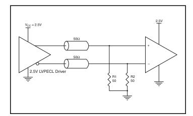
Figure 4C. 2.5V LVPECL Driver Termination Example
