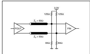
Figure 3B. 3.3V LVPECL Output Termination
