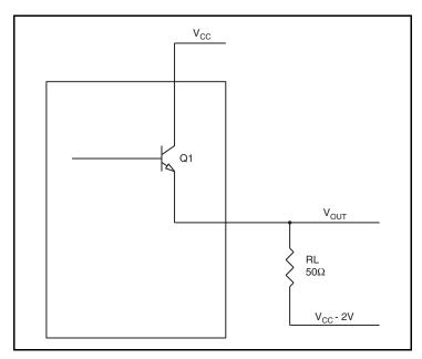
Figure 5. LVPECL Driver Circuit and Termination
