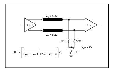
Figure 3A. 3.3V LVPECL Output Termination
