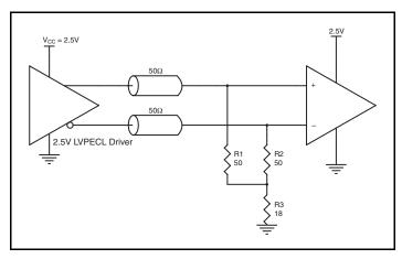
Figure 4B. 2.5V LVPECL Driver Termination Example
