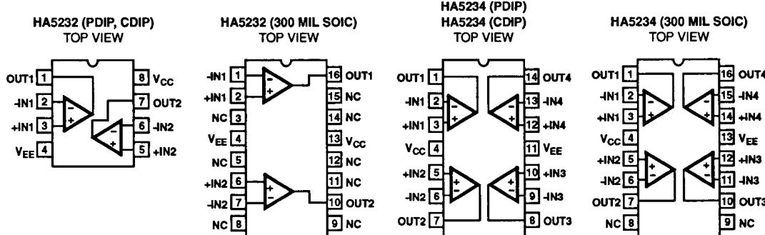
NOTE: The functional pinouts will comply to the JEDEC standards for dual and quad op amps as shown above
