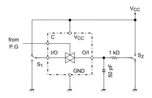
2. Cross Talk (control input-switch output) fIN = 1 MHz duty = 50% tr = tf = 6 ns
