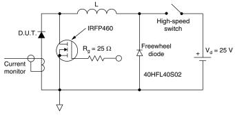
Fig. 8 - Unclamped Inductive Test Circuit
