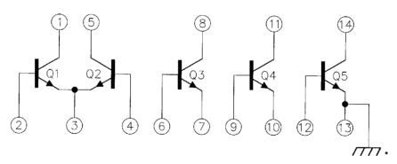
\* Substrate pin must be connected to the most negative DC potential - which should also be a good AC ground - for proper isolation between transistors.
