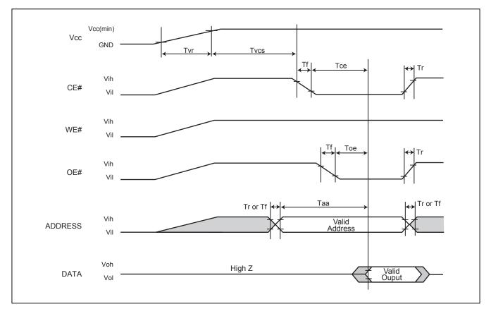
Figure A. AC Timing at Device Power-Up
