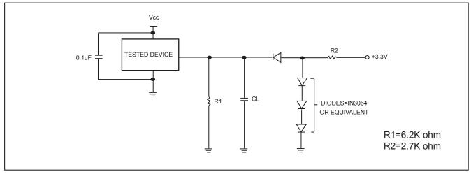
Test Condition Output Load : 1 TTL gate Output Load Capacitance,CL : 30pF(70ns)/100pF(90ns) Rise/Fall Times : 5ns In/Out reference levels :1.5V
