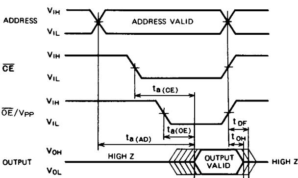
Test conditions for AC characteristics
