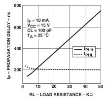
Figure 9. Propagation delay vs. load resistance
