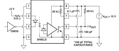
Figure 15. Optocoupler input to output capacitance model for shielded optocouplers
