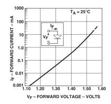
Figure 4. Input current vs. forward voltage
