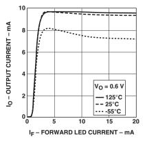
Figure 1. Typical transfer characteristics
