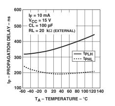
Figure 7. Propagation delay with external 20 k $\Omega$  RL vs. temperature
