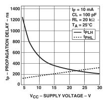
Figure 11. Propagation delay vs. supply voltage
