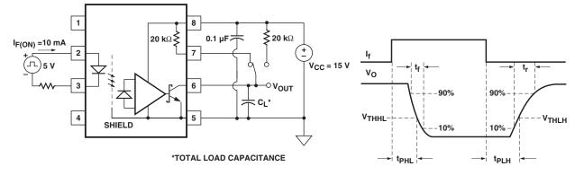
Figure 5. Propagation delay test circuit
