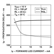
Figure 12. Propagation delay vs. input current
