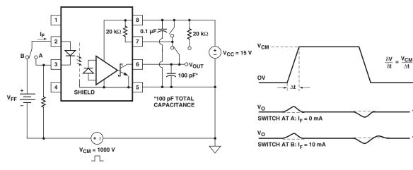
Figure 6. CMR test circuit. Typical CMR waveform
