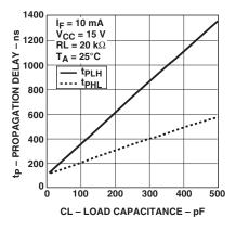
Figure 10. Propagation delay vs. load capacitance
