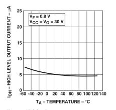
Figure 3. High level output current vs. temperature
