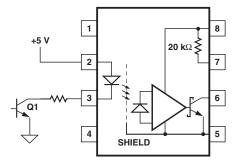
Figure 19. Not recommended open collector LED drive circuit
