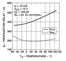
Figure 8. Propagation delay with internal 20 k $\Omega$  RL vs. temperature
