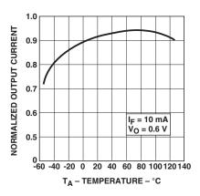
Figure 2. Normalized output current vs. temperature
