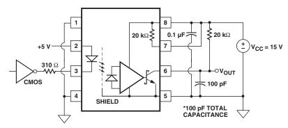
Figure 13. Recommended LED drive circuit
