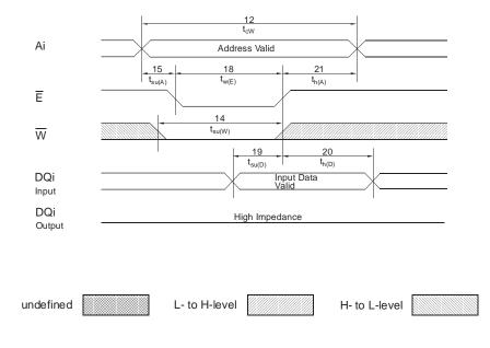
i: If  $\overline{W}$  is low and when  $\overline{E}$  goes low, the outputs remain in the high impedance state.
