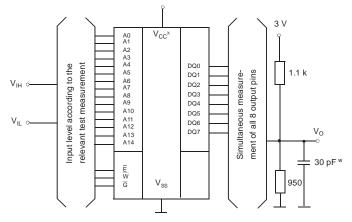
w: In measurement of  $t_{\rm dis}\text{-times}$  and  $t_{\rm en}\text{-times}$  the capacitance is 5 pF.
