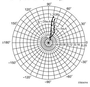
$\begin{array}{l} S21e:V_{CE}{=}10V\\ f{=}100MHz,\,200\;to\;1200MHz(200MHz\;step) \end{array}$
