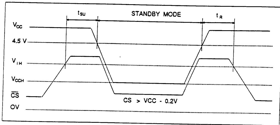
**LOW  $V_{CC}$  DATA RETENTION CHARACTERISTICS**
