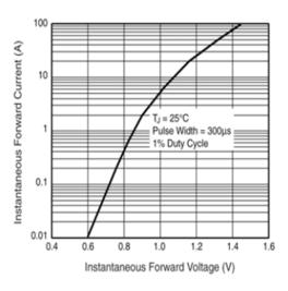
Figure 3. Typical Forward Characteristics Per Leg
