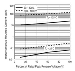
Figure 4. Typical Reverse Leakage Characteristics Per Leg
