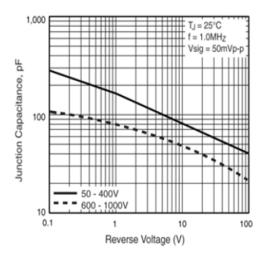
Figure 5. Typical Junction Capacitance Per Leg
