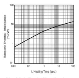
Figure 6. Typical Transient Thermal Impedance
