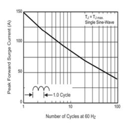
Figure 2. Maximum Non-Repetitive Peak Forward Surge Current Per Leg
