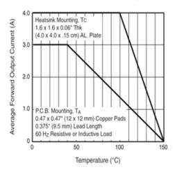
Figure 1. Derating Curve Output Rectified Current
