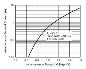
Fig. 3 - Typical Instantaneous Forward Characteristics
