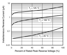
Fig. 4 - Typical Reverse Characteristics
