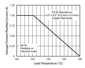
Fig. 1 - Forward Current Derating Curve
