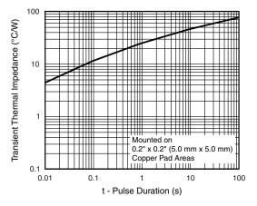
Fig. 6 - Typical Transient Thermal Impedance
