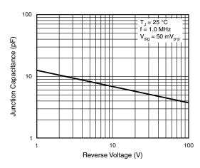
Fig. 5 - Typical Junction Capacitance
